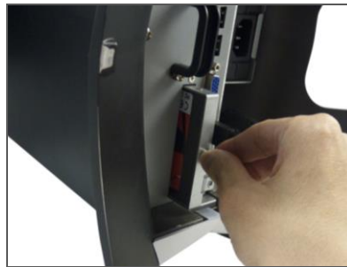
Simple 1-Screw HDD Replacement
