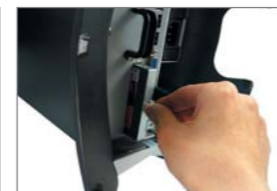
Simple 1-Screw HDD Replacement
